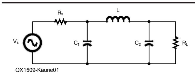
Figure 1 — This schematic diagram shows a low-pass pi network.
